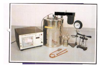
Provided simple and inexpensive method for determination of heat of combustion of Organic matter and the calorific value & sulpher contents of solid & liquid fuel. The outfit is supplied complete for analysis as per the method recommended by BS 1016/. All parts of the outfit are machined as per the specifications.
